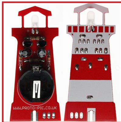
**Step 6:** We now need the power switch, don't worry about which way around this goes, simply pop it in the holes at the bottom, solder it up and trim the pins and it should look like this:
