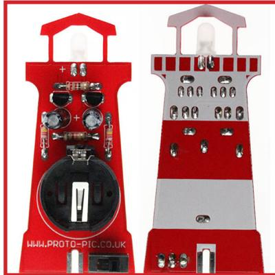
**Step 7:** Finally we're almost done! now all you need to do is slot the base into the bottom of the light house and solder the two together. Soldering one or two joins should be more than enough to keep it together. When soldering it lay the whole thing on it's side and solder them like this:
